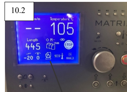
Paper sensor signal for no paper
