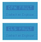
When the sensor is in open circuit, **OPN FAULT** displays on the LCD.
