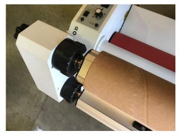
Now attach the Media brackets and mandrel with the 4 remaining screws into the 2 screw holes towards the back of the machine:
