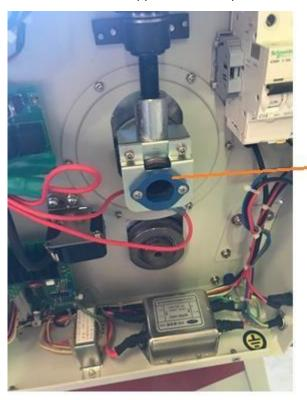
Rubber Support For Element Remove the Green Rubber sleeve on the left and right sides and attach the wire to each end of the element, ensuring there is a washer on either side of the terminal as shown in the pictures below.
