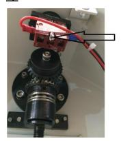
Take off the emergency stop button by unscrewing the screw above.
