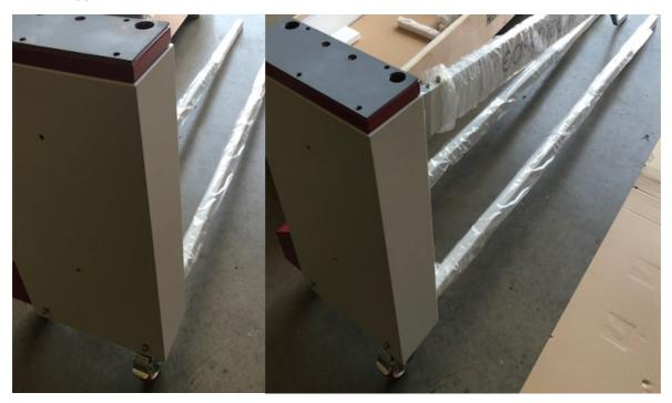
Put the Right Stand Frame on and secure using 6 x Stand Bolts.
