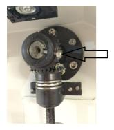
Untighten the screw above to loosen the bevelled gear.
