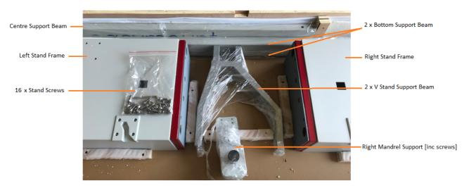
Attach the 2 x V Support Beams to the Centre Beam as in the below picture using 8 x Stand Bolts.
