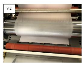
9. Manually push the feed roller down and insert another card (9.1). While pushing the card press the foot pedal, moving the sheet into the rollers until it reaches the feed gate (9.2). Put on the safety guard and push in the latch (9.3).
