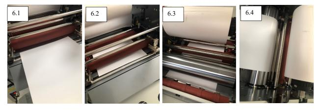
6. Place a plain thick (i.e.300gsm) card into the back of the machine (6.1) taking care to go the middle of every roller (6.2) until reaching the feed gate (6.3), then place another plain card and cover the top laminating roller (6.4).
