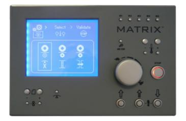
As explained on previous page press the function/settings key to enter screen, use the temperature buttons to select mode and press stop to enter.
