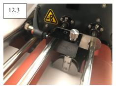
12. Set the guide wheel in the centre of the sheet (12.1). Set the perforator – ensure the perforator wheel is in line with the film (up to 5mm) and within the media crop lines. Once aligned tighten the perforator into position using the black handle (12.2), then turn the silver threaded thumb screw clockwise to lower the perforator wheel (12.3). Too much pressure will perforate through the paper.
