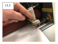
13. Set the angle wheel on the edge of the print inline with the perforator and tighten the black handle (13.1) – set a small amount of angle and tighten the top black handle (13.2). Different paper stock requires different pressure of the angle wheel, this can be adjusted using the silver knurled knob (13.3), clockwise will increase the pressure.
