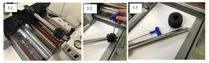
3. Remove film mandrel off the system and loosen the core collar using the blue 5mm Allen key provided (3.3)
