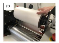
8. Drape the film over the chrome roller and feed table (8.1). Push a plain thick card in-between the chrome roller and feed roller (8.2), while pushing the card through turn the film clockwise to release the tension (8.3). Push the card until the back edge is inline with the feed gate (See below figure 9.1).
