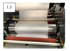
1. Ensure the display anti-curl setting is set to zero (1.1), enter the display double sided mode (1.2) (page 7-8 for display navigation) and turn on the bottom roller temperature (set at minimum of 10 degrees higher than the top roller). Remove safety guard (1.3).
