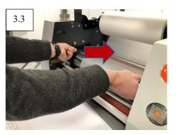
3. Remove both silver thumb screws (3.1), pull the handles inwards and towards the roller (3.2). The edge closest to you of the feed gate plate should come out first (3.3). Remember which way it comes out as it can only go back in the same way.
