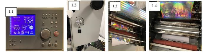
1. Enter the foiling mode (1.1) (for display navigation on page 7), put the express idle bars on the machine (1.4) and turn the take up on to setting one (1.2). Put on the express foil kit idle bars on the front and rear of the system (1.3).
