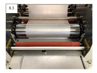
8. While pushing the card press the foot pedal (8.1)l, moving the sheet into the rollers until it reaches the nip (8.2) and put the feed gate plate and thumb screws back into position (8.3).
