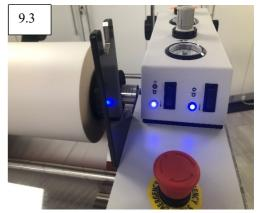
9. Put the safety guard back on ensure the latch is pushed in (9.2), otherwise the eye on the display will flash and the machine will not run. Lower both pneumatic laminating roller and pull roller (the LED's will illuminate blue when the roller is in the down position - figure 9.3).
