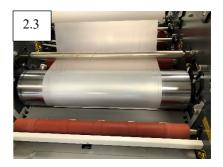
2. Press the forward foot pedal key and select 0.5mmpm speed (2.1). Press the foot pedal (2.2) until the sheet edge is in the nip of the laminating rollers (2.3), ensure you can still see the paper as to avoid getting glue on the bottom roller.
