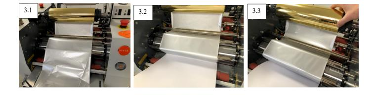
3. Thread the foil under the patterned idle bar and drape over the top laminating roller including the express foil kit idle bars (3.1). Push a plain thick card in-between the chrome roller and feed roller (3.2), while pushing the card through turn the foil clockwise to release the tension (3.3). Push the card until the back edge is in line with the feed gate (4.1).
