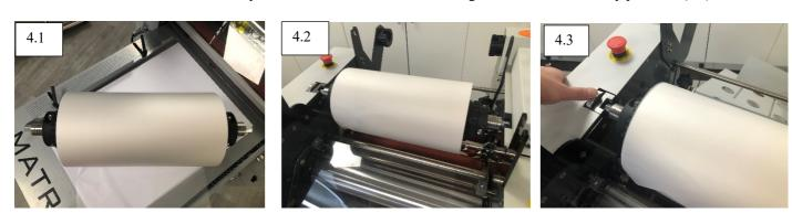
4. Slide film onto the mandrel and centralize (4.1). Replace the core adaptor and tighten. Place the mandrel back onto the system and tighten the mandrel lock (4.3).
