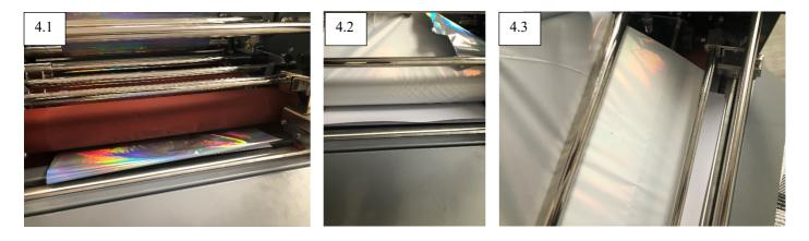
4. Thread the foil in-between the angle wheels and perforator support bars (4.2), under and around the rear express kit idle bar (4.3) and attach the take up unit as shown below (4.4). Select the temperature and pressure required, lower the laminating roller pressure and put the safety guard on. When foiling we do NOT need the pull roller, this must remain in the up position (4.5).
