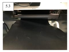
5. Push the feed sheet down until it reaches the bottom foam idle bar and thread around the back (5.3). Pull towards the front of the system and load bottom roll of film. Ensure this is centralized and matches the top roll of film. The bottom film is a mirror image of the top. The adhesive should always face you when pulling of the roll (5.4).
