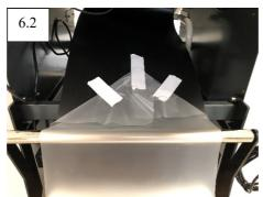
6. Fold the film over on itself and secure it to the feed sheet (6.1). This needs to be as flat as possible (6.2). Slacken the film to the floor to allowing enough to pull the feed sheet out of the system (6.3).
