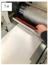
7. Pull the feed sheet up onto the feed table (7.1) and remove. Cut the film to leave a clean edge (7.2) and stick it to the top laminating film (7.3). Manually push the feed roller down and insert a thick 300gsm plain card (7.4).
