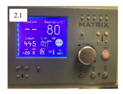
2. Set paper length (exclude the desired overlap i.e. 450gsm = 445mm) and set temperature to 80°C.
