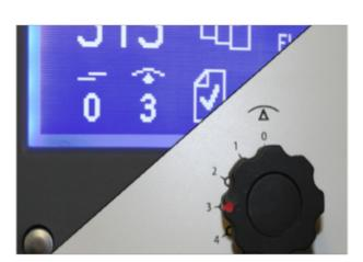
Ensure the perforator wheel is set over the laminating film within 5mm from the edge and anti-curl mechanical setting matches the display setting. Depending on the media and material being used you might require both angle wheels, ensure the angle wheel on the left is angled more than the one directly next to the perforator. If you have Pneumatic splitting pressure this might need to be increased, for single sided is usually between 0.2-0.4psi and double sided between 0.4-0.6psi.
