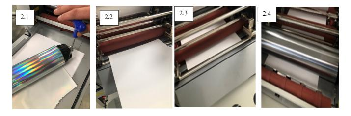
2. Put the foil onto the mandrel (2.1), ensure it feeds from the bottom of the roll, place a plain, thick (i.e.300gsm) card into the back of the machine (2.2) taking care to go the middle of every roller (2.3) until reaching the feed gate (2.4).
