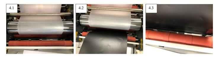
4. Push the feed card down in between the bottom laminating roller and grey support plate (4.2 & 4.3). Ensure the Matrix Duplex writing is facing the feed table (see below 5.1 & 5.2).
