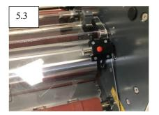
5. Ensure the film feeds from the bottom (5.1) of the roll and mechanical anti-curl is set to zero (5.2). Remove safety guard (5.3).
