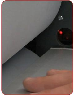
You can adjust the rate at which the machine laminates by turning the 'speed control knob' up to a maximum of 6m/min.
