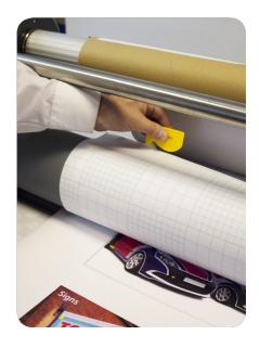
Select foot pedal mode and select a slow speed, then press the foot pedal and inch the laminate through the rollers until the cut backing paper faces you.
