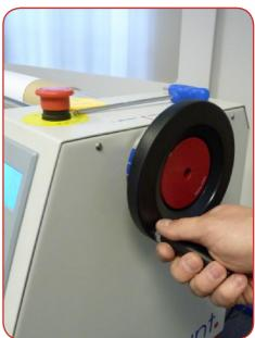
The media will then correct itself and run through smoothly. Film running loose and climbing up onto the take up core. This occurs when there is <u>NO</u> tension added to the film.
