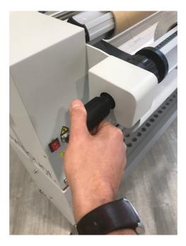
Pull the laminate from the back of the machine in the centre of the laminate with one hand while lowering the top roller with the other hand.
