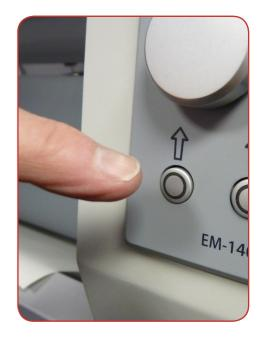
The films will then begin to be drawn through the machine. NOTE: When using continuous mode if the 'magic eye' sensor is blocked by material or hands the machine will stop, to override the sensor press the foot pedal.
