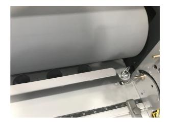
Higher the roller and pull the laminate through the machine.
