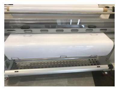
The Laminate should be tensioned enough to prevent creases on the media, if the laminate is following the backing paper either reduce the tension on the backing paper or increase the tension on the laminate.
