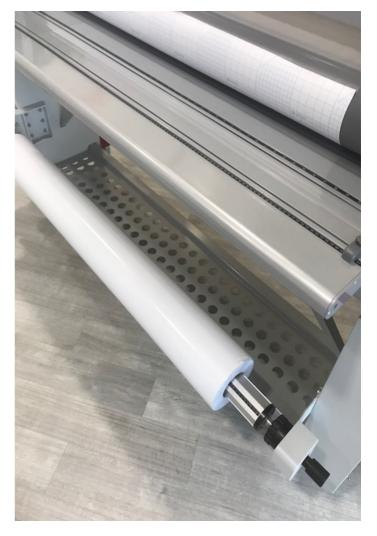
Lift the feed table in the up position and secure remaining media to the film, higher the top roller and insert the vinyl around the threading bar into the rollers.
