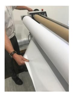
Once film is held in place separate the backing paper from the film using the safety knife provided.
