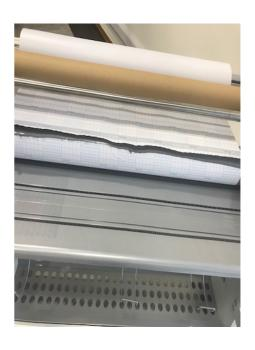
Pull the backing paper up towards the take up mandrel from the centre and secure it to the core using packing tape in 3 places, the centre, left and right.
