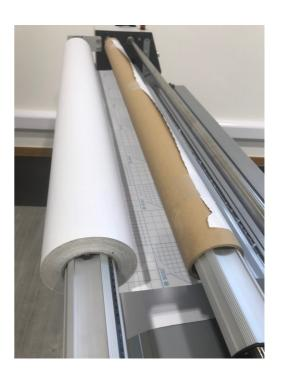
Pull the remaining backing paper of the laminate down to the feed table and roll your vinyl and place in the hooks provided.
