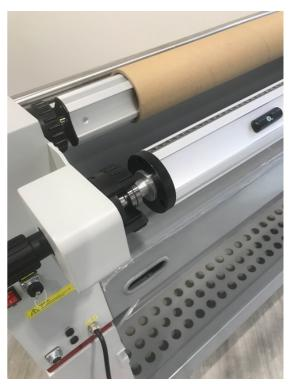
Pull out the Swing out arm and slide the laminate in place.
