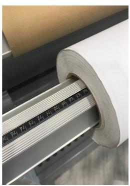
Remove the take up mandrel [waste mandrel] by opening both locking sleeves and slide on a 3 inch core, then lock the mandrel back into place.
