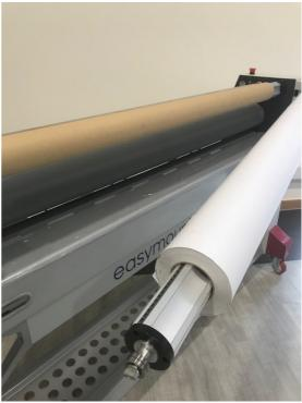
Locate the swing out arm back into its home position & centralize the laminate on the mandrel using the measurement guide.
