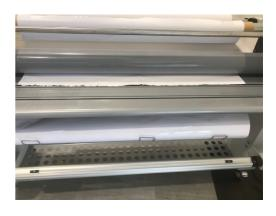
Insert the media support plate and safety guard. Feed your media over the feed table and into the nip of the rollers.
