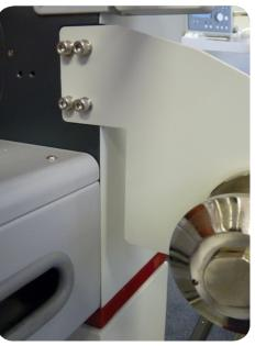
Plug in the take up unit. Select full speed, forward & combine. Fit the take up mandrel (note the bracket is sprung loaded on the motorised unit). Then using double sided tape attach media/laminate to the core, the Easymount laminator is now ready to run prints reel to reel.
