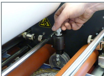
20. Turn the screw as the paper is feeding until the perforation wheel starts to turn, then lock into position.
