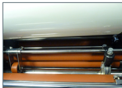
21. Set the guide wheel to the opposite side of the sheet from the perforation wheel.
