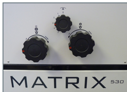
18. Lower the laminating and pull rollers and set the anti-curl to the desired setting - suggested starting position 2-3, if the print curls up increase the anticurl number, if down decrease.
