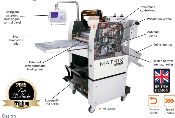
The Matrix Duplex is an incredibly cost-effective system that allows printers to laminate single-side, double-side and encapsulate their work, in-house.
