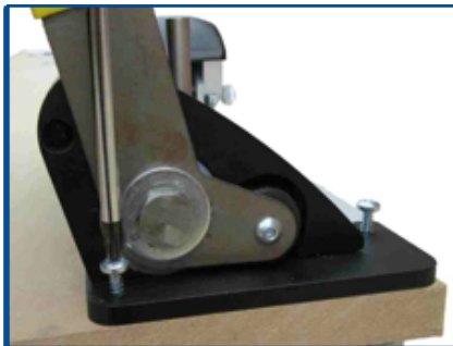
5. Attach the two end plates to the table using the pan head screws provided. Check that each lifting handle operates correctly.
