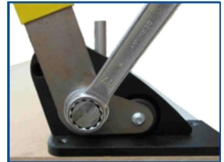
3. Using a 17mm spanner, fit a lifting handle to each end. Once tightened, the handles should move freely without any sideways movement.
