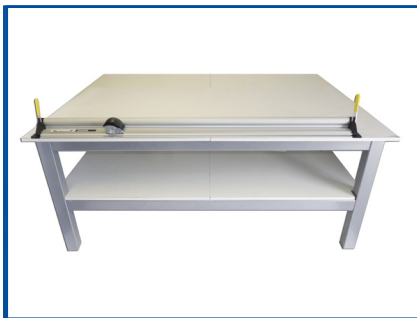
4. Check that the cutter is in the correct position on the table and check that the base plate and end plates are in line.
