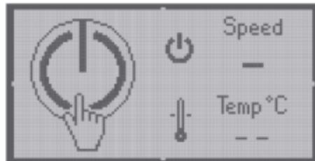
Waking up from the Standby mode. Press the button again. The blue backlight is ON, and the laminator starts Warming Up Clock and revert to the last setting used.
