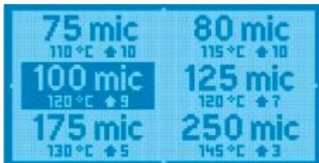
Press either Temperature Adjustment Button or Speed Adjustment Button, the laminator turns into Manual Mode, and the Hand Symbol will show on the display. In Manual Mode, you can adjust the speed value or temperature value according to the pouch film
