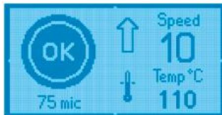
The Thickness of Pouch Film (B): In Preset mode, the thickness of pouch film will show on the display.
