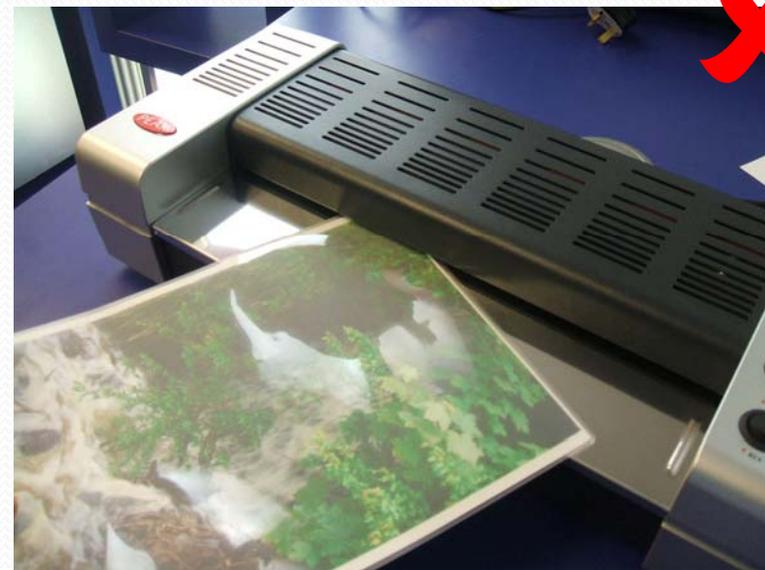
Remember to always insert your document with the sealed end first. This is very important so that the laminator does not jam.
