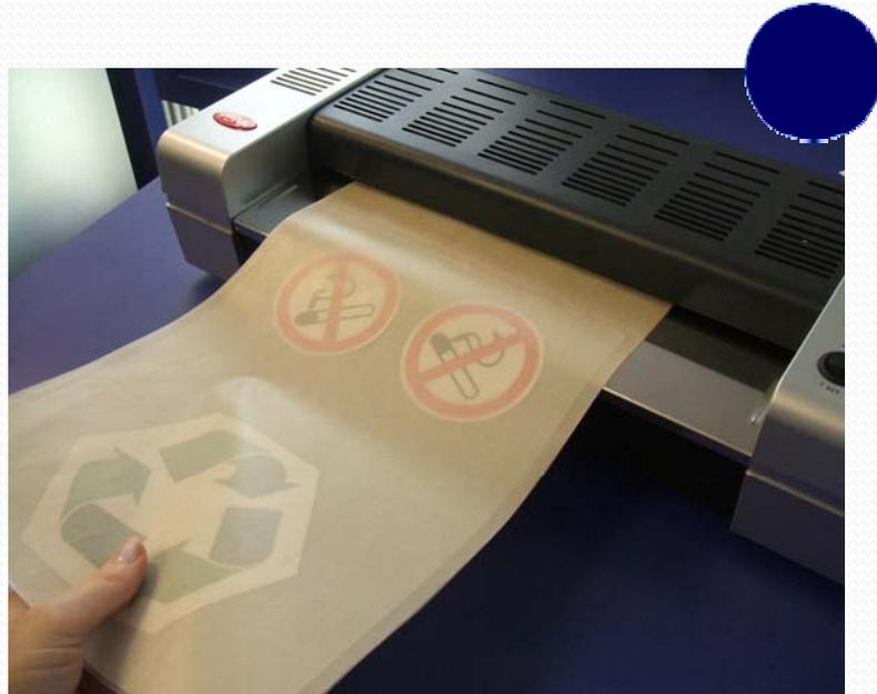
Once you have finished all of your laminating work, turn your heater button to OFF and allow the laminator to run for 5 minutes to allow it to cool down. After this time it is safe to turn your POWER switch to OFF.
